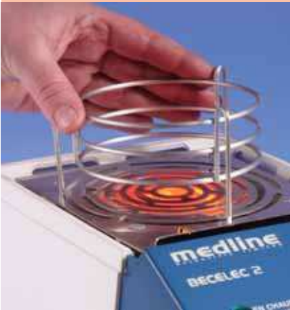
The wire safety guard (included) adds to the safety aspect of this burner.
